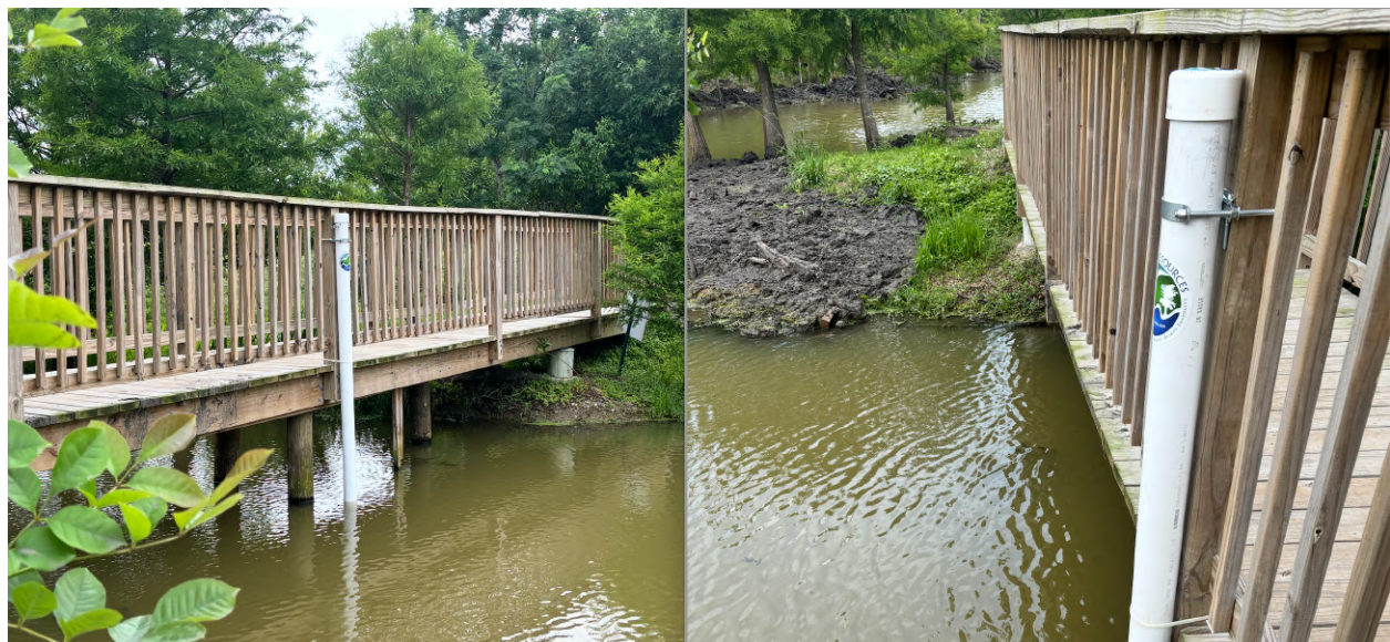
The housing holding an Aqua Troll 600 multiparameter probe on May 28, 2026.
